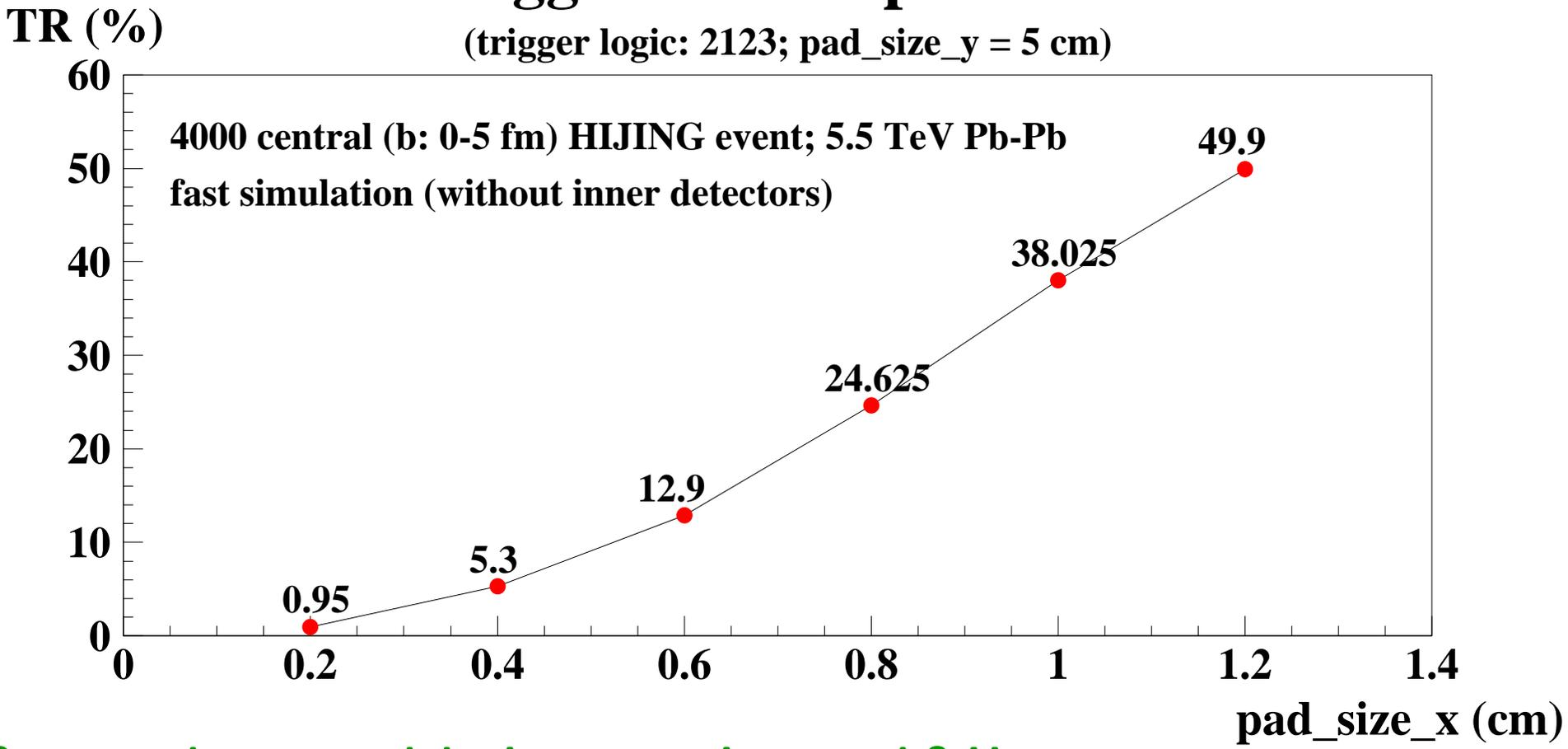
With 2 mm pads one modul trigger rate is around 8 Hz.
