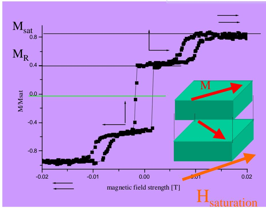
Magnetization loop at 260K of the trilayers TG= 575K. The value of the remanence ( $M_R$ ) is half the saturation value, consistent with a 90° alignment of Fe layers.
