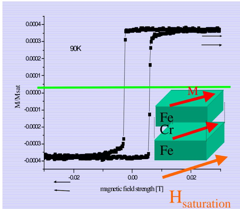
Magnetization loop at 90K of the trilayer Fe/Cr/Fe grown at 575K (ferromagnetic).
