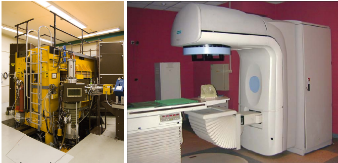
Figure 17.51: Left: Cyclotron used in medicine to produce radioactive isotopes. Right: Linear accelerator used in a hospital
