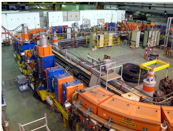
Figure 17.6: The Low Energy Ion Ring (LEIR) at CERN. The Pb ions are collected and stored in the ring while continuously cooled. The pipes of the stochastic cooling are above the ring. The electron cooling is set up on left: the two guns are for introducing and removing the electron cloud. The bending magnets are painted orange, the quadrupole doublets and triplets blue. LEIR uses the elements of the former Low Energy Antiproton Ring (LEAR) functioning in 1982–1996
