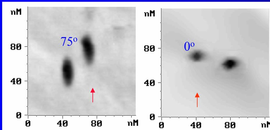
AFM phase images of  $\alpha\text{-Al}_2\text{O}_3$  surfaces irradiated with 710 MeV Bi ions. Arrows show the ion beam direction
