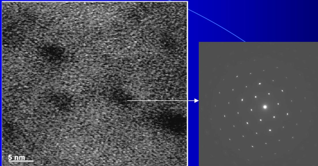
High-resolution lattice image of  $\alpha$ - $A_2O_3$  irradiated with 710 MeV Bi ions a fluence of  $7 \times 10^{12} \text{ cm}^{-2}$  at room temperature (plan-view specimen). The average TEM track diameter is  $\sim 3$  to 4 nm.
