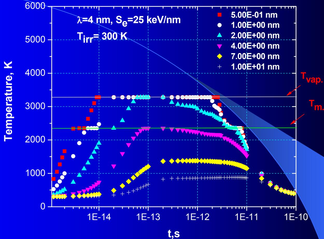
Temperature evolution at different radial distances from the Bi ion axis in sapphire.  $T_m = 2340 \text{ K}$ , vaporisation temperature is  $3280 \text{ K}$ .  $\lambda$  - electron-lattice interaction mean free path (calculated with TSPIKE02 code. *M. Toulemonde, C. Dufour, A. Meftah, E. Paumier, Nucl. Instr. and Meth., B 166–167 (2000) 903.*
