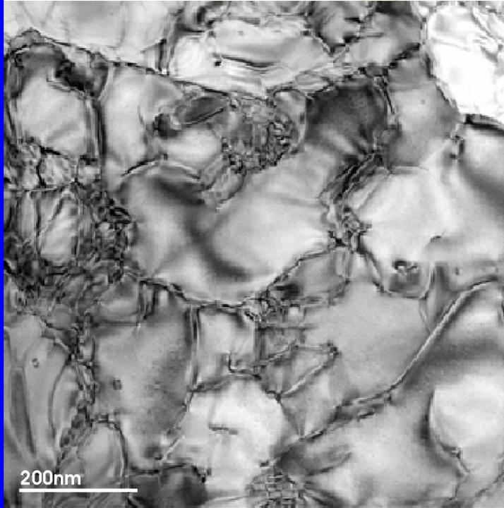
TEM micrograph of  $\alpha$ -A<sub>2</sub>O<sub>3</sub> target irradiated at  $S_e=41$  keV/nm to a fluence of  $7 \times 10^{12}$  cm<sup>-2</sup> (S.J.Zinkle, ORNL)
