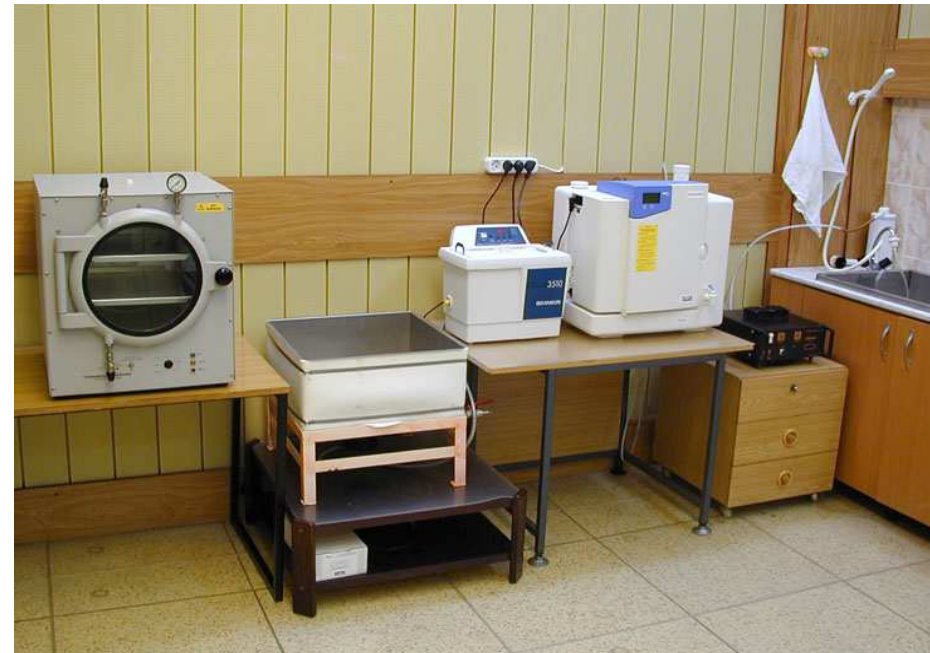
Figure 2: vacuum furnace ( Vacu Heat 17 L (200 C 9) ), water purifying system ( Purelab Option – S7 (7,5 l/h) ) and ultrasonic bath ( ИЛ100-5 (39x37x14 cm) )
