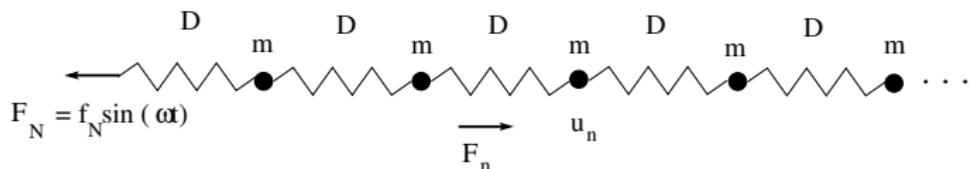
$$\begin{aligned} m a_n &= -F_n + F_{n-1} \\ F_{n-1} &= -D(u_n - u_{n-1}) \end{aligned}$$
