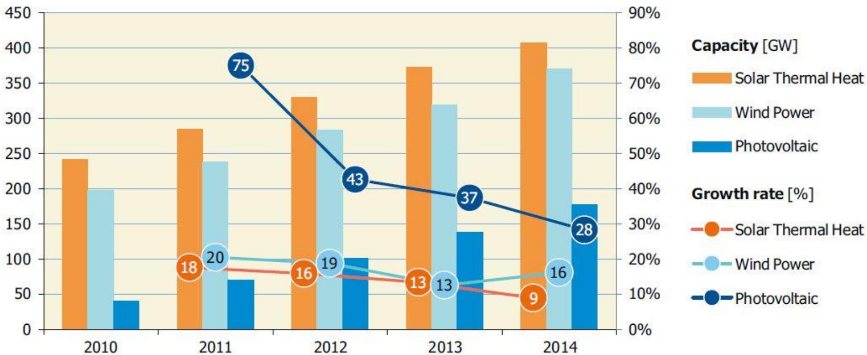
Figure 4: Global solar thermal heat, wind power and photovoltaic capacity in operation and market growth rates between 2010 and 2014
