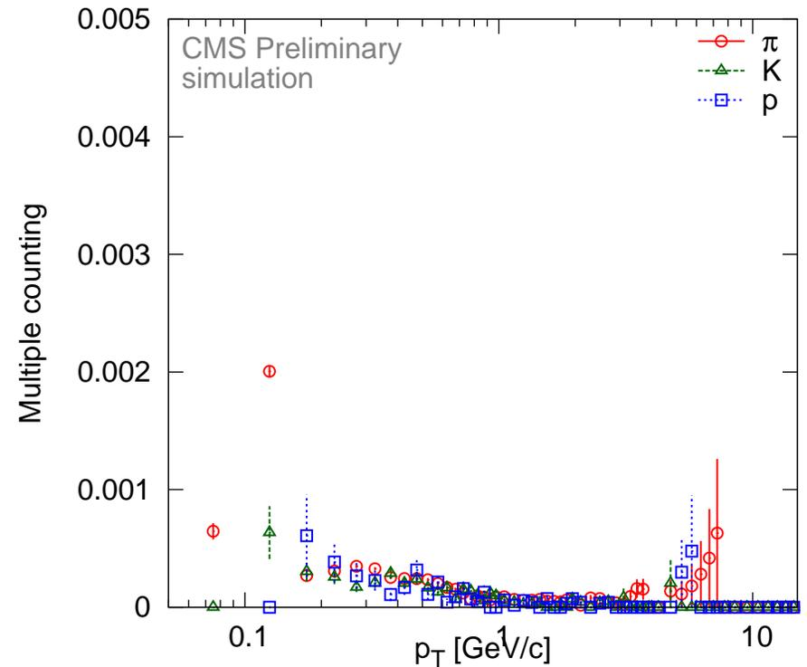
Fraction of reconstructible particles which are more than once reconstructed
