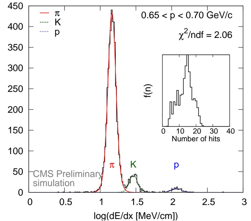
Combined fit using sum of many gaussians, where  $\sigma \propto 1/\sqrt{n_{\text{hits}}}$
