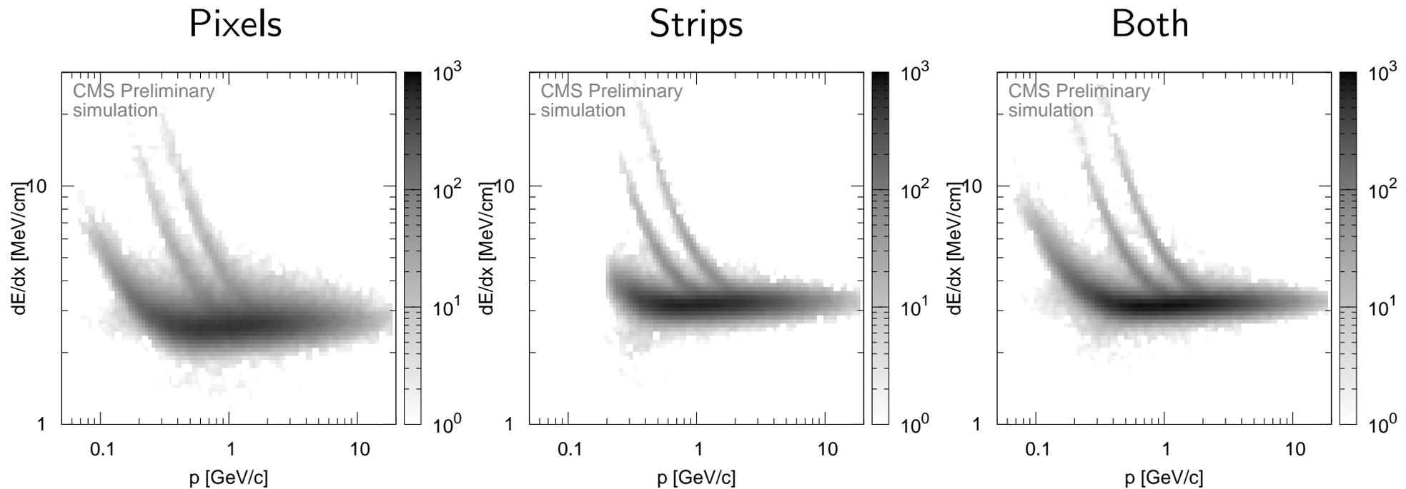
Truncated mean  $dE/dx$  (average of lowest half) using both pixel and strip hits
