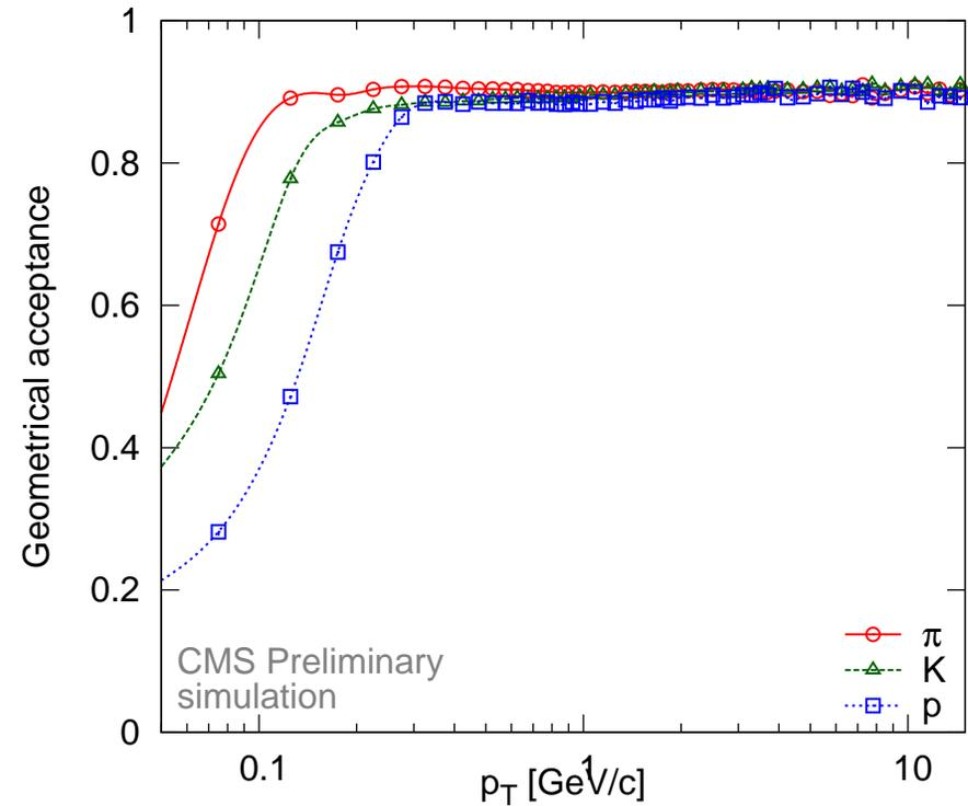
Fraction of simulated particles which are reconstructible
