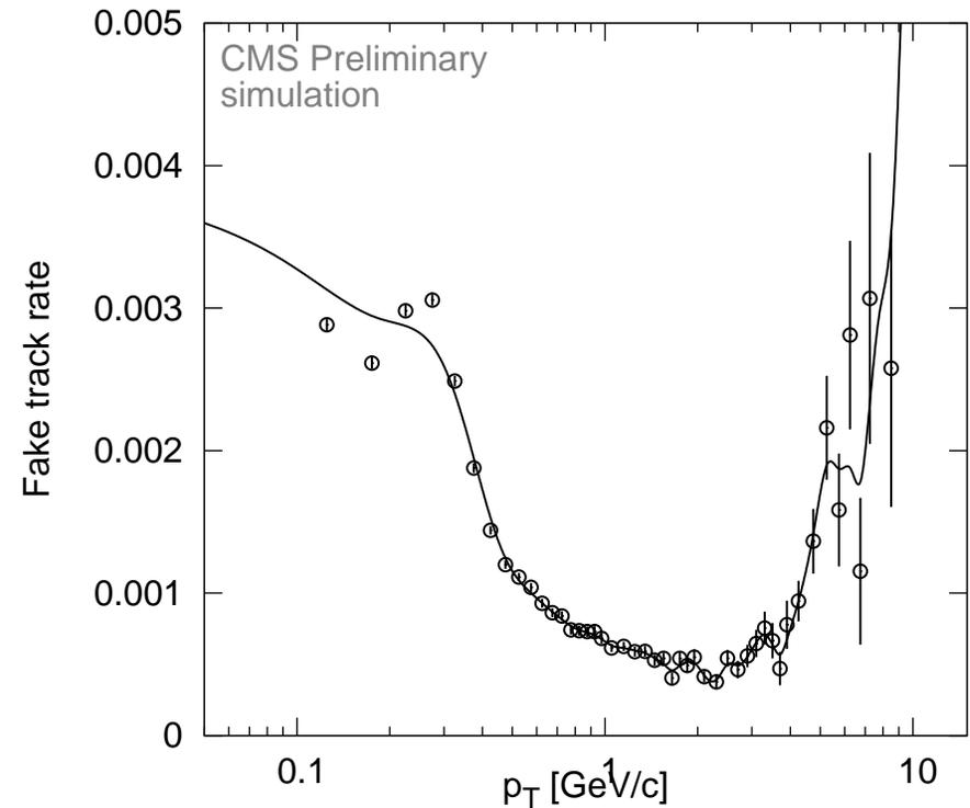
Fraction of reconstructed tracks which are fake
