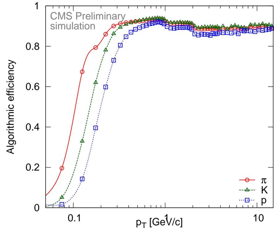
Fraction of reconstructible particles which are at least once reconstructed
