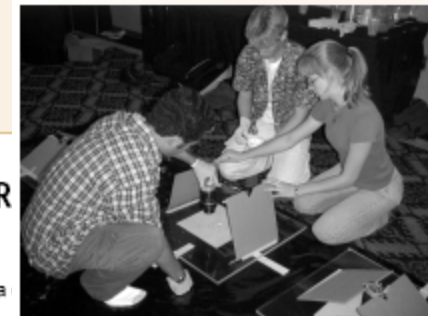
SALTA students gluing photomultiplier tubes to scintillator panels at the Snowmass workshop.
