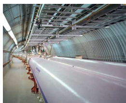
RHIC's rings consist of 1,740 superconducting magnets.
