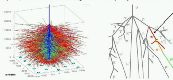
Showers are detected by large lateral coverage ground detector arrays.
