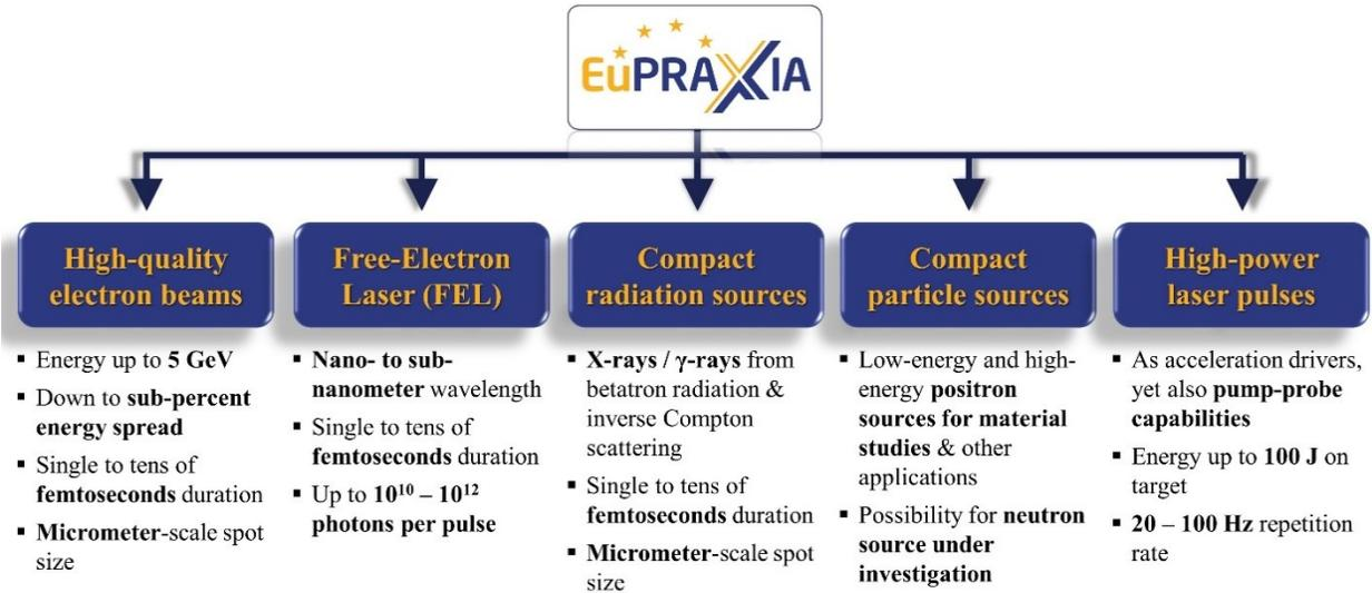
**FIGURE 2:** Main goals foreseen for the future EuPRAXIA facility layout and beamline properties. A more finalized and detailed description of the facility and the provided beam parameters will be available in October 2019 in the EuPRAXIA Conceptual Design Report.
