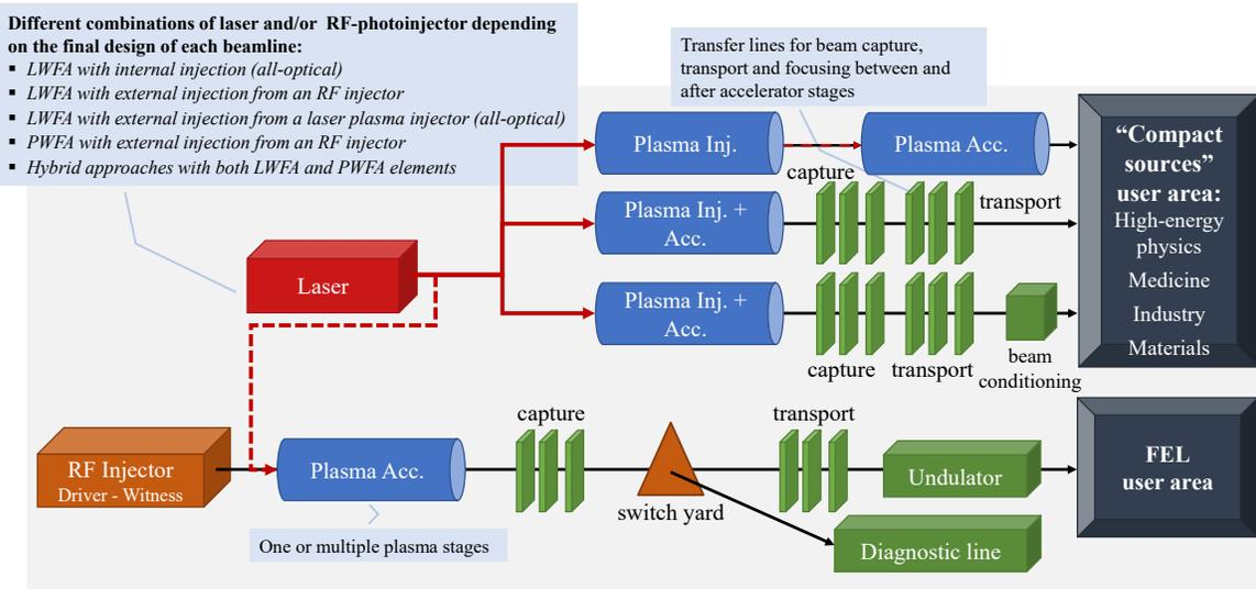
**FIGURE 1:** Overview over an exemplary EuPRAXIA beamline setup with its main elements and some of the design choices (such as injection and acceleration technique(s), number of beamlines and end station design) still under investigation. A final beamline layout will be presented in the EuPRAXIA Conceptual Design Report in Oct 2019.
