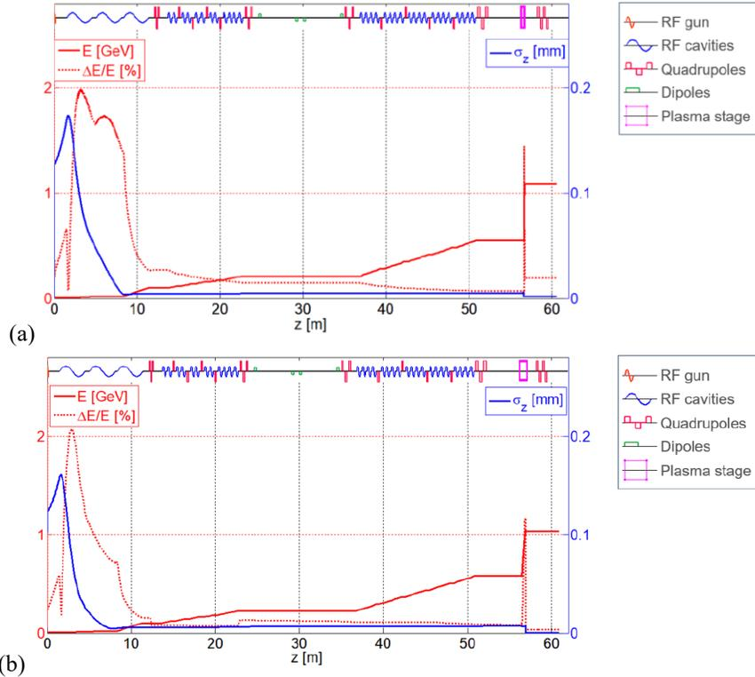
**FIGURE 3:** Start-to-end simulations for the witness electron bunch after acceleration using a laser-driven wakefield accelerator (Fig. (a), LWFA) and using a beam-driven wakefield accelerator (Fig. (b), PWFA). The electron bunch energy (red), relative energy spread (red dotted) and bunch length (blue) are shown in each case. Details of these simulation studies can be found in reference [31], from which these images are reproduced with permission of the authors.
