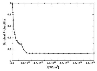
**Fig. 1.** Stabilization of the potassium atom in a superatomic field: survival probability vs. laser intensity for a 800 nm, 65 fs laser pulse. For details, see reference [30].
