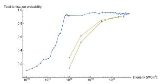
Fig. 2. Total ionisation probabilities as a function of the laser intensity.  $\lambda = 800 \, \text{nm}$ ,  $\tau = 120 \, \text{fs}$ . The blue line corresponds to the ab initio calculations, the orange and the green to CTMC simulations with the model potentials (30) and (31), respectively.
