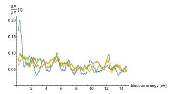
**Fig. 3.** Energy spectrum of the continuum electron. The blue, orange and green lines are for  $I=10^{12}, 2.5\times 10^{13}$  and  $8.1\times 10^{13}\,\mathrm{W\,cm^{-2}}$ , respectively.
